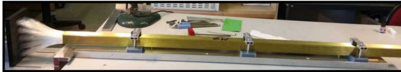
Central tower loaded with fibers
